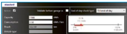
Figure 4 Parametrization of GENIOS's e-bus optimization module. The parameter can be adjusted on-the-fly and allow for comparison of different scenarios.
